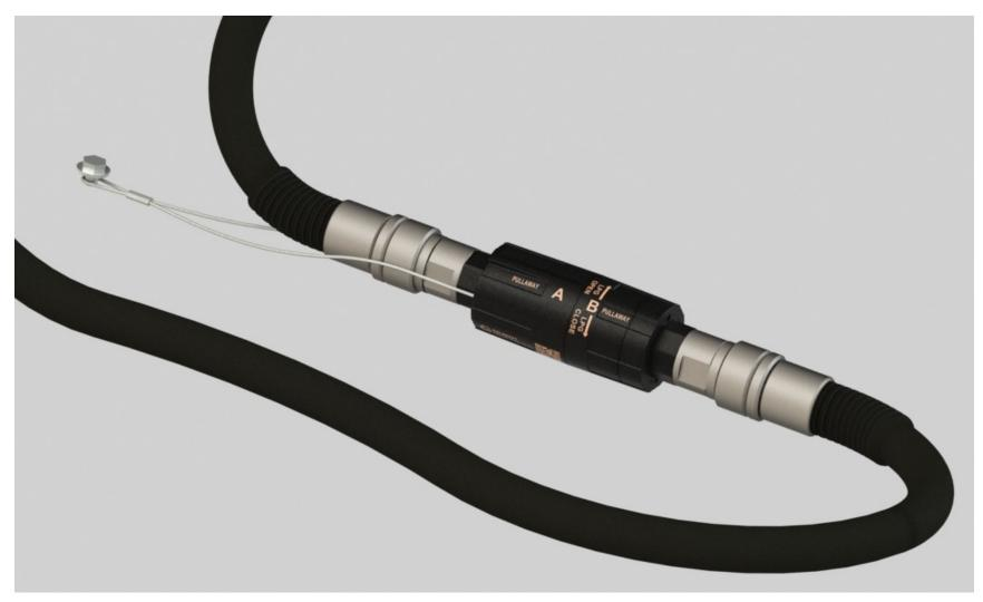
The Pullaway consists of two main parts: a fixed part that is hooked to the ground (A) and a movable element that disengages if excessive traction is exerted on the tube (B).
