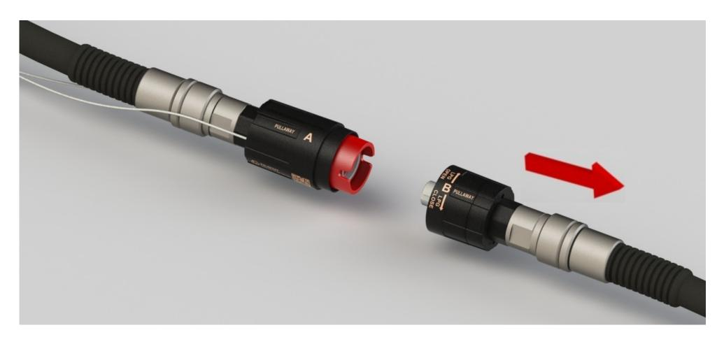
If excessive traction is exerted on the hose, the Pullaway intervenes by disengaging, preserving the integrity of the dispenser.
